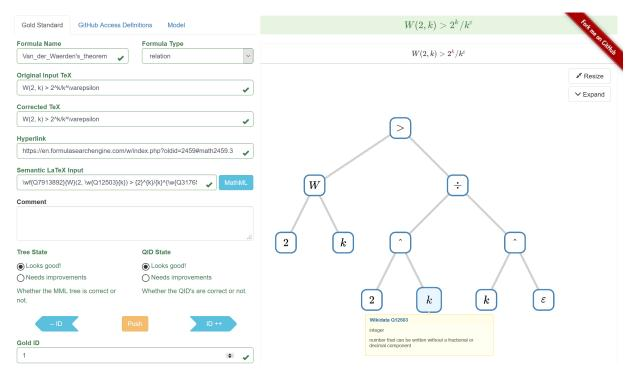
Figure 1: Graphical user interface to support the creation of our gold standard. The interface provides several TEX input fields (left) and a mathematical expression tree rendered by the VMEXT visualization tool (right).
